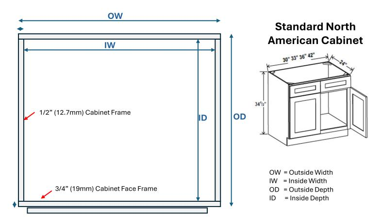
Can be adjusted to fit within a Width Cabinet of 24", 28", 30", 34", 36", 38", 40", & 42" cabinet base.
