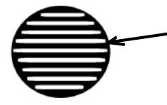
Vents are on the underside of the units, which allows the fans to properly vent and cool down the system from below, which look like this image. 2 Burners will have 1 vent, 3 and 4 Burners will have 2 vents and 5 Burner will have 3 vents that must not be obstructed.
